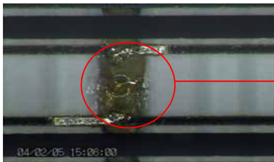
Panel electrode Insulation break down
